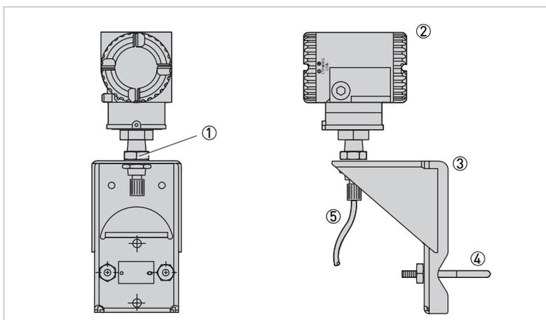
Figure 3-12: Mounting the remote electronics housing
