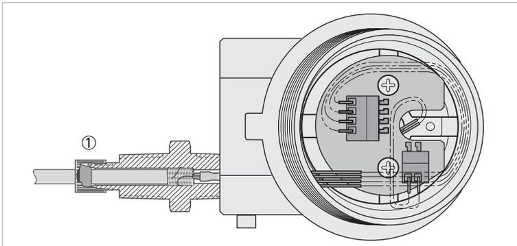
Figure 4-1: Connecting the remote signal cable
