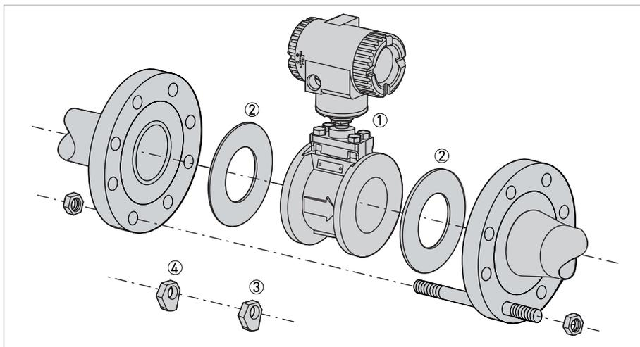
Figure 3-10: Flowmeter centering using spacers
