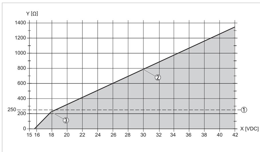
Figure 4-4: Relationship of output load versus supply voltage
