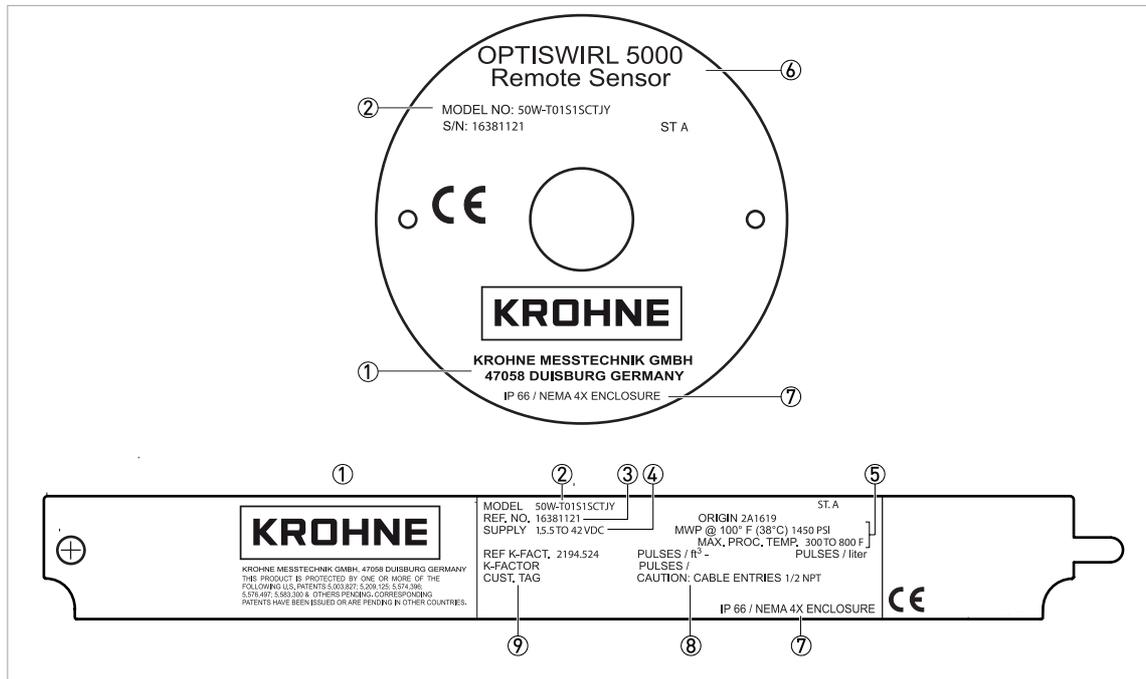
Figure 2-5: Example of a nameplate for the remote version
