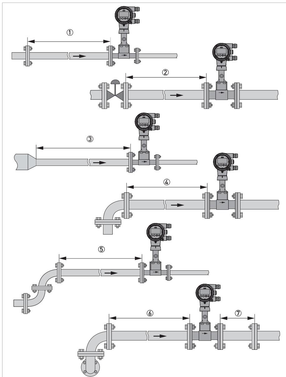
Figure 3-6: Minimum inlet sections
