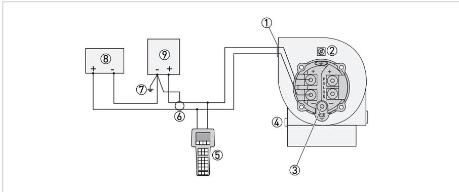
Figure 4-5: Wiring a flowmeter with a 4...20 mA output
