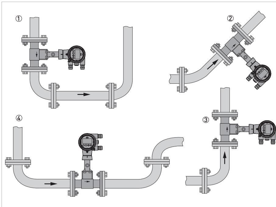
Figure 3-1: Recommended installation
