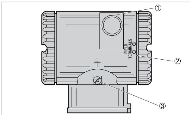
Figure 4-2: Access to flowmeter field terminals
