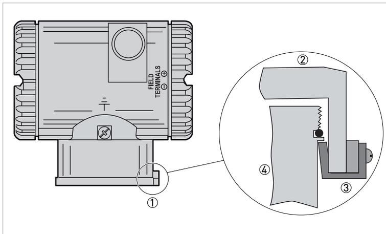
Figure 3-15: Turning the connection housing
