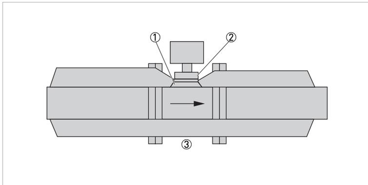
Figure 3-13: Installation heat insulation
