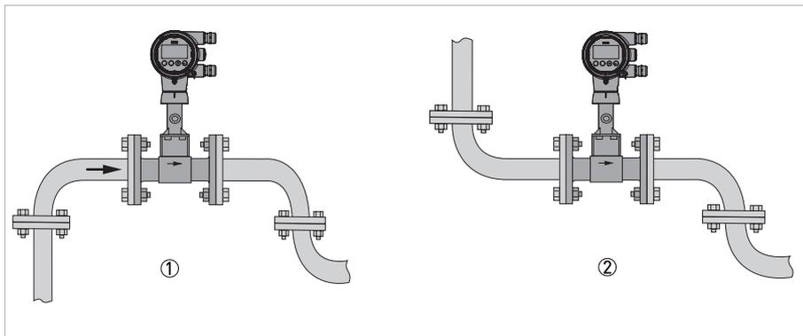
Figure 3-3: Recommended installation
