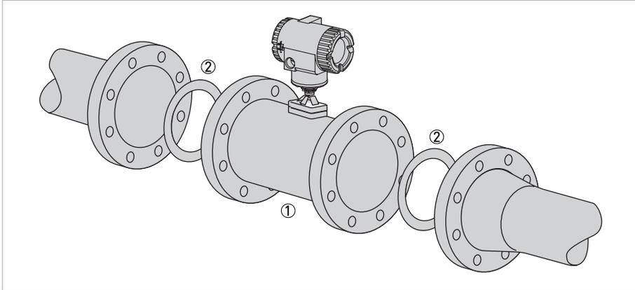
Figure 3-11: Installing devices in flange design
