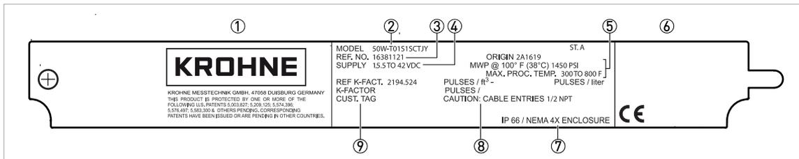
Figure 2-4: Example of a nameplate for the compact version
