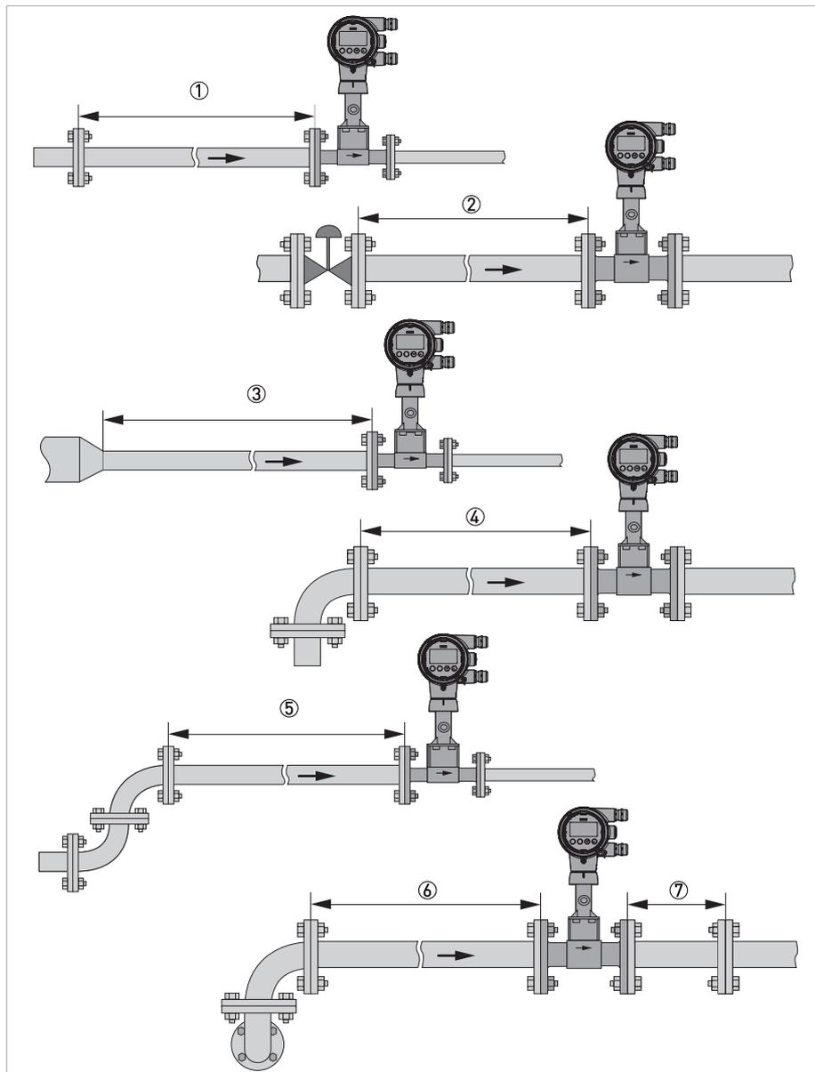
Figure 3-6: Minimum inlet sections
