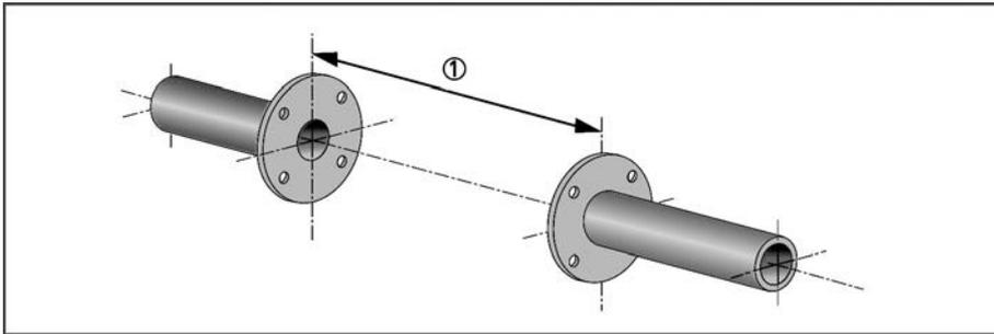
Figure 3-8: Preparing the metering point
