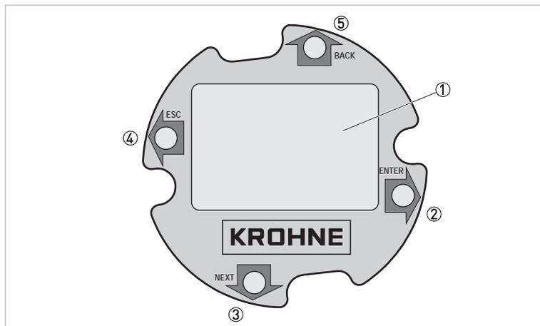
Figure 5-1: Description of local keypad/display
