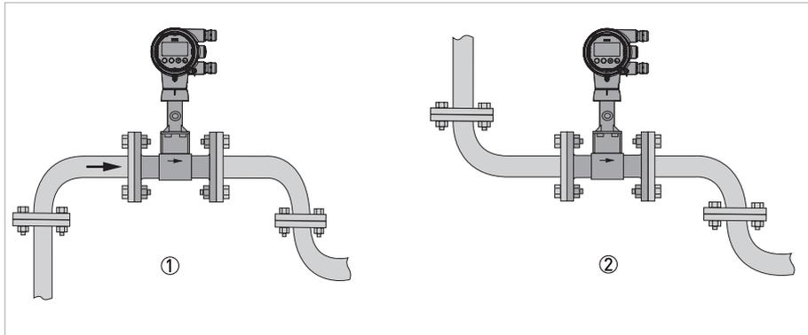
Figure 3-3: Recommended installation
