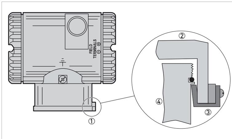
Figure 3-15: Turning the connection housing
