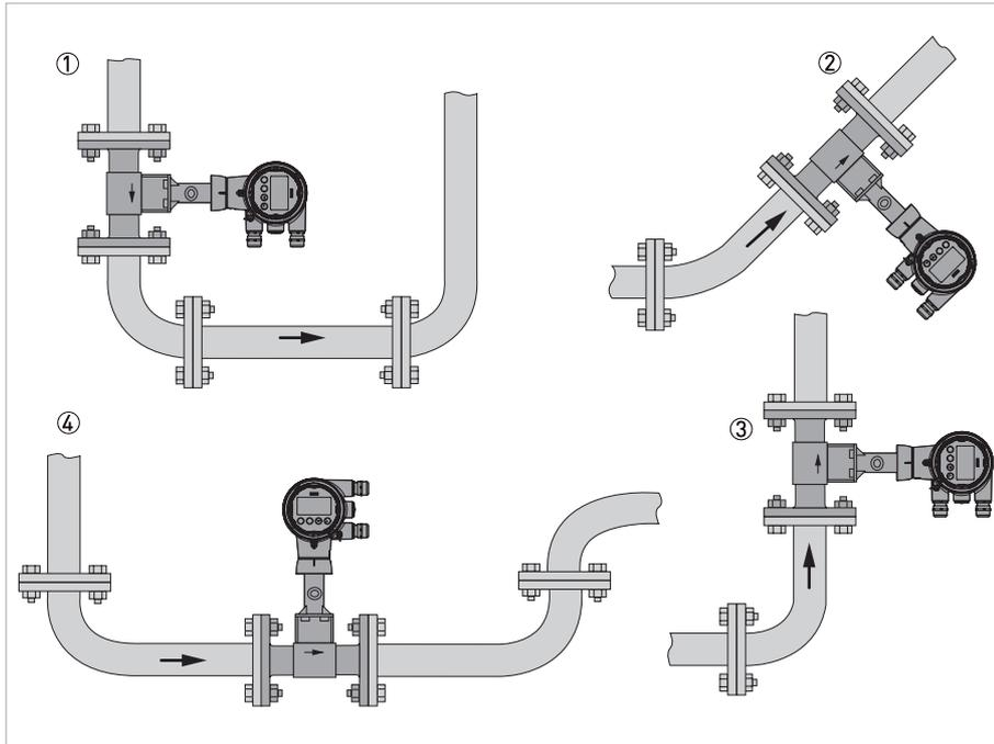
Figure 3-1: Recommended installation
